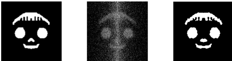
Fig. 4 Synthetic object, H^{-1} applied to the real projection , computed solution.
