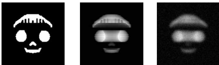
Fig. 1 Synthetic object, theoretical projection Hf , real projection with noise and blur.
