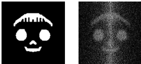
Fig. 2 Comparison between the real object on the left-hand side and the reconstruction computed with H^{-1} applied to the real projection on the right-hand side.
